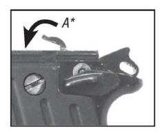
The ejector should be depressed <u>only</u> far enough to provide clearance for the slide during assembly. Depressing the ejector beyond the point required for reassembly <u>may</u> cause the ejector to bind in the frame. Should this occur, the ejector will not return to the normal position. This condition is not correctable at the operator level - the pistol will have to be returned to SIG SAUER for repair.
