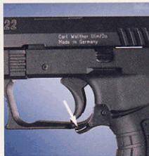
Magazine Release Molded to the same contour as the trigger guard, prevents the magazine from being unintentionally released from the weapon. The ambidextrous magazine release can be operated equally well by either right or left-handed shooters.
